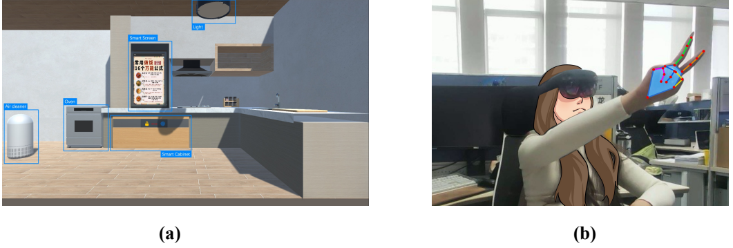
Fig. 11. The experimental platform utilized in the smart home scenario. (a) IoT device control interface, simulated using Unity. (b) User wearing the HoloLens and performing gestures with the right hand for device control.
